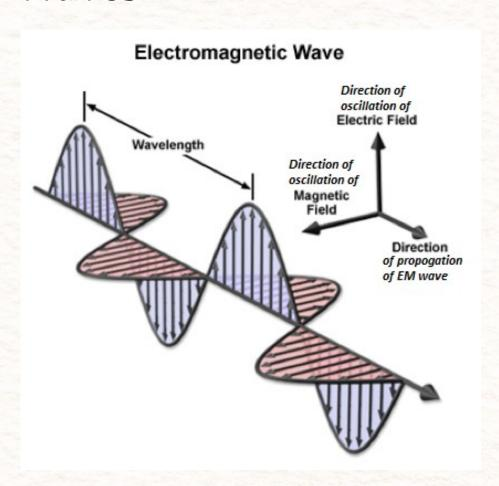
Radio signals are transmitted by an Electromagnetic Wave
