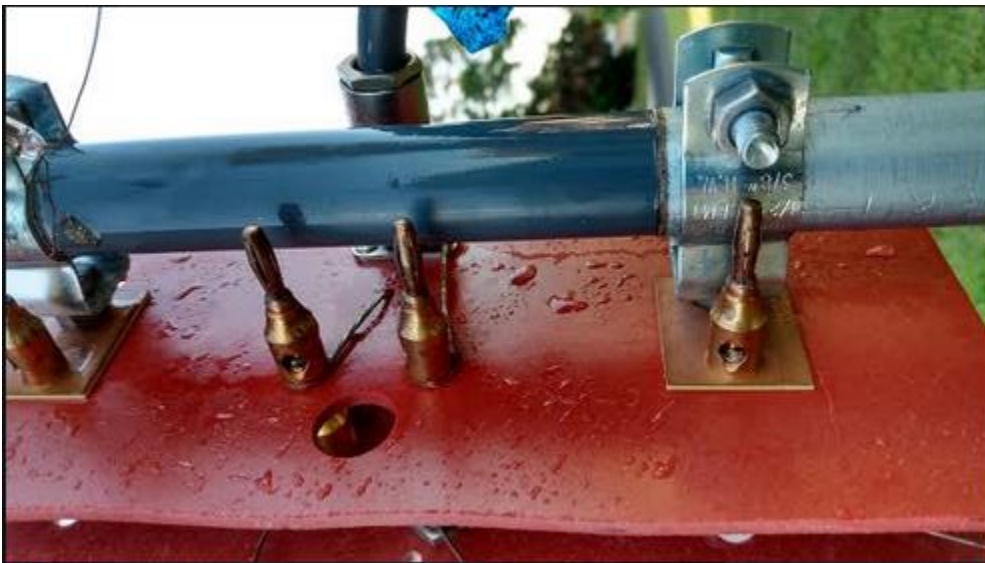
Back side of mounted mother board. Wire was used for connection of the SO239 to the center receptacles. Small pieces of copper clad board or brass sheet were used to connect the ends of the loading coils to the antenna mounts. View rotated 90 degrees
