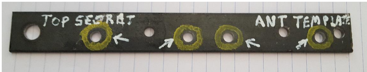
A Top Secret steel template for locating holes.
