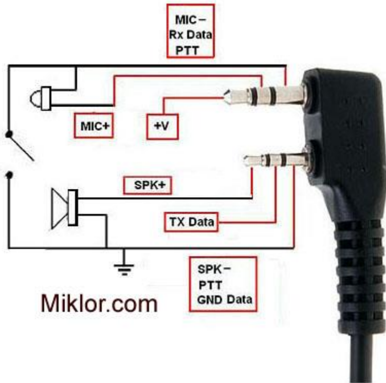
Kenwood style speaker/mic pinout
