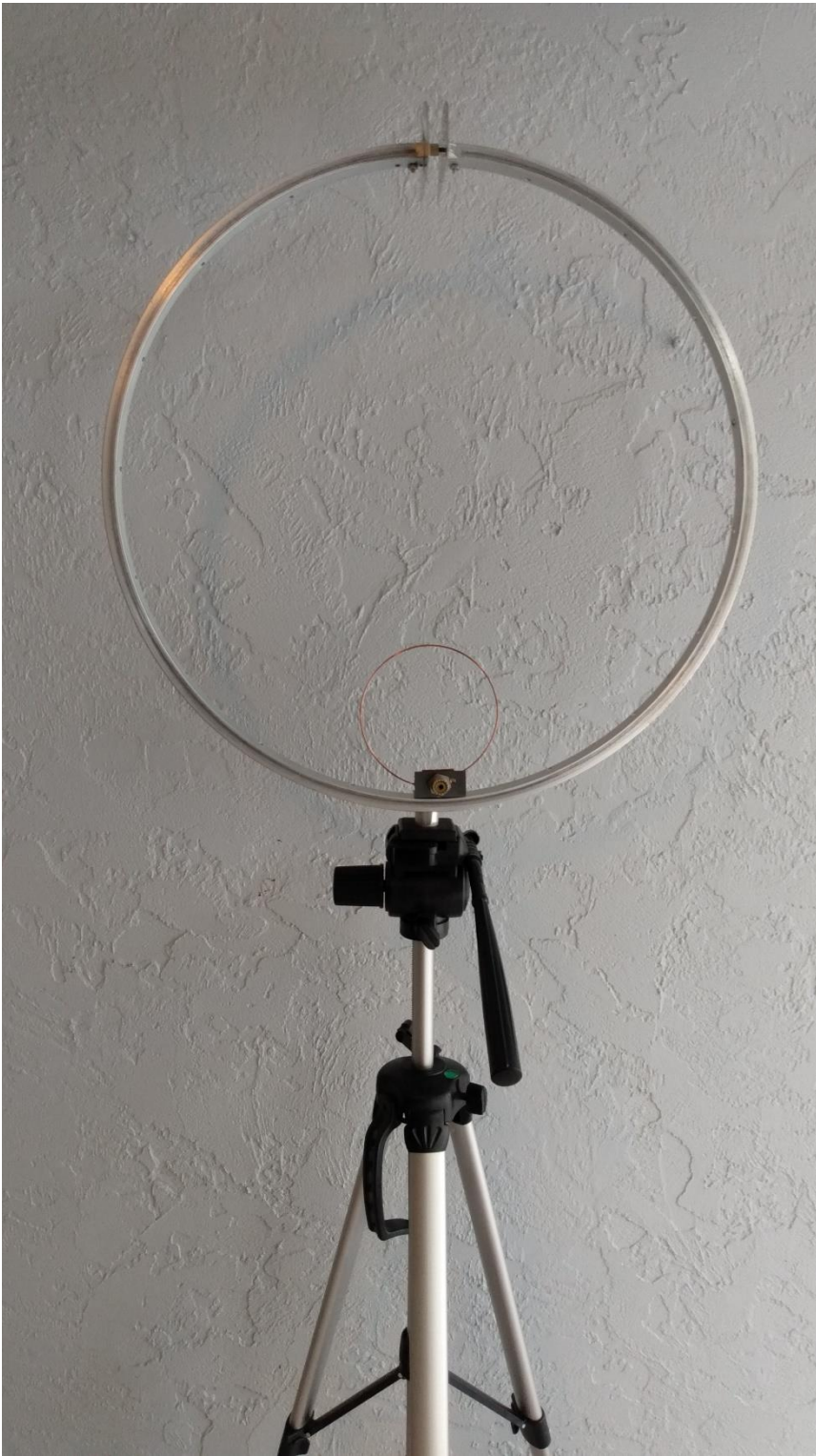
6M bicycle wheel mag loop antenna
