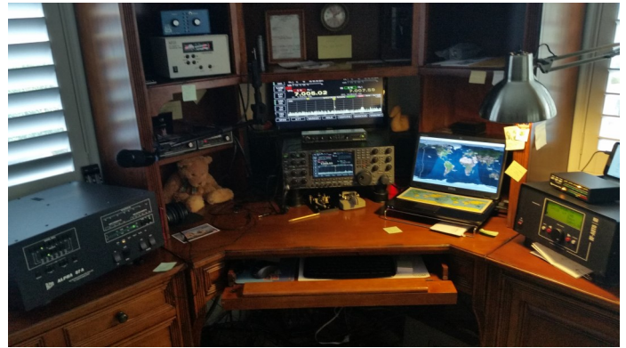
^Station #5 is Bob's main station powered by an Icom IC 7800 160-6M into an Alpha 87 A 1.5 kW amp with a Pal Star HF 2kW auto-tuner. A straight key, keyer, and seldom used mike provide interface. Rotor control is switchable remotely from here and other stations.
