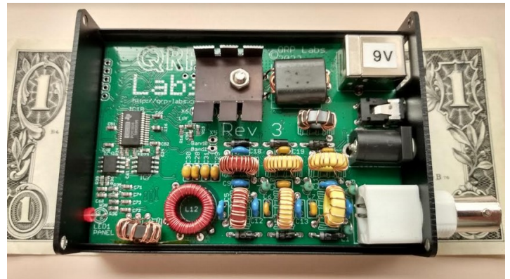
The assembled QDX. All surface mount components are preinstalled.
