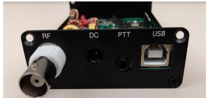
The assembled QDX. All surface mount components are preinstalled.
