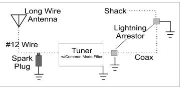
I followed that idea and put one on the #12 antenna wire before the tuner input insulator. To do so I used a small piece of copper plumbing tubing, threaded it with a spark plug tap, lightly hammered it on top of the ground rod, screwed the plug into it using some copper thread anti-seize compound, then put the ground clamp around it to secure it to the rod. I connected the antenna wire to the plug using an electrical connector I found at Home Depot.
