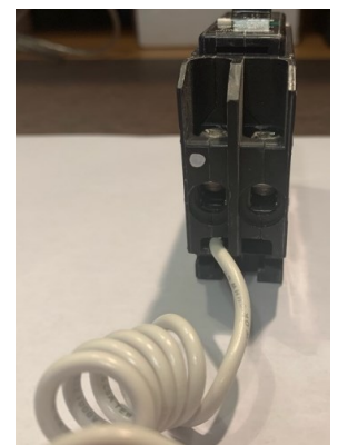
Eaton AFCI - note the two terminals, the one with the white dot is for the neutral. The pigtail goes to the neutral bar in the breaker box.
