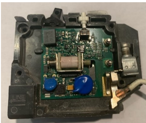
Eaton AFCI internals showing the processing electronics and the solenoid that trips the breaker
