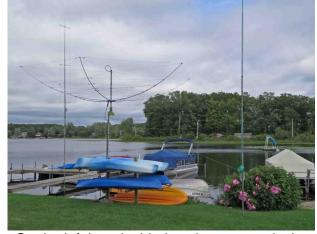
On the left is a double-bay 6-meter vertical antenna. In the center is Stan's new Hex Beam mounted on a 10 ft pole. The mast on the right supports a 40m, 30m, 20m, 15m dipole. After the operation, the Hex Beam was moved to a 48' self-supporting tower at Stan's QTH.
