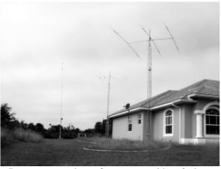
Dan uses a variety of antennas, with a 3-element tribander at 30', a 4-element beam for six meters, a 13-element beam for two meters, and a vertical for 10-40 meters. A good basic ham radio set up.
