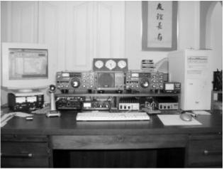
Again, Dan uses vintage Yaesu equipment, running 200 watts on 6- and 2-meter Phone and CW.
