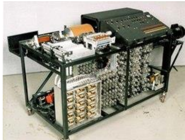
The Atanasoff-Berry computer used racks of vacuum tubes.
