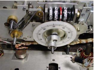
Here's a close up photo of the planetary gear drive for the rotary dial frequency display, which is calibrated in kHz, and the rotary drum dial for determining the MHz. Note the continuous ball chain, operated by the band selection control, which drives the drum dial frequency display and the components of the slug tuners in the RF section.
