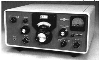
The 51S-1 is a dual or triple conversion (dependent on the frequency) USB, LSB, AM, and CW receiver for signals from 0.2 to 30.0 MHz. Coverage is continuous in thirty 1-megahertz bands. The 51S-1, and its variants, utilize 17 tubes and 12 semiconductors. It was introduced in 1959 at a price of \$1828 (about ½ the price of a new '59 Ford convertible), primarily for the military and commercial market. Used ones are currently fetching \$1100-2100.
