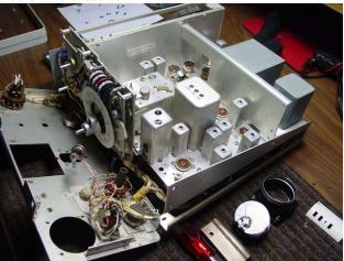
The above photo shows more of the main chassis layout, with the power supply and audio sections located behind the aluminum RF shield.
