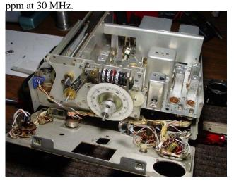
The previous photo shows the chassis of Bob's 51S-1, stripped of its tubes, meter, etc. Note the wiring harness, and the beautiful finish on the aluminum chassis even after years of service.
