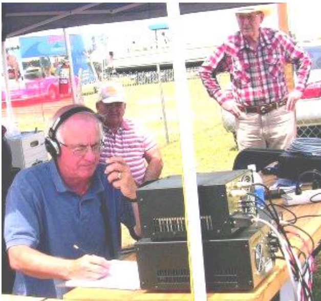
Here's Andy-KB1HIP handing out the QSOs on the last day. That's Andy's solid state Ameritron amp on top of the IC-746PRO, and that gain in signal was a big boost to the QSO rate.
