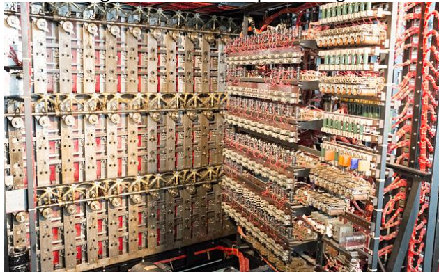
A replica of the Turing Bombe machine, used for cracking German military Enigma codes, at Bletchley Park
