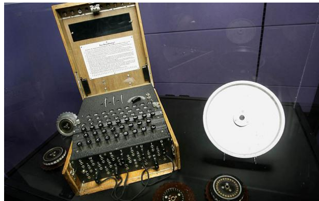
A 1935 Enigma machine, used by Germans to encrypt messages during World War II
