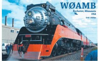
Built by Lima (Ohio) Locomotive Works in May 1941, 4449 is the only surviving Southern Pacific GS-4 class of steam locomotives. The locomotive is a streamlined 4-8-4 (Northern) type locomotive. She operated in California until retired in 1956. Fully restored in 1974, she operates on excursion services to this day.
