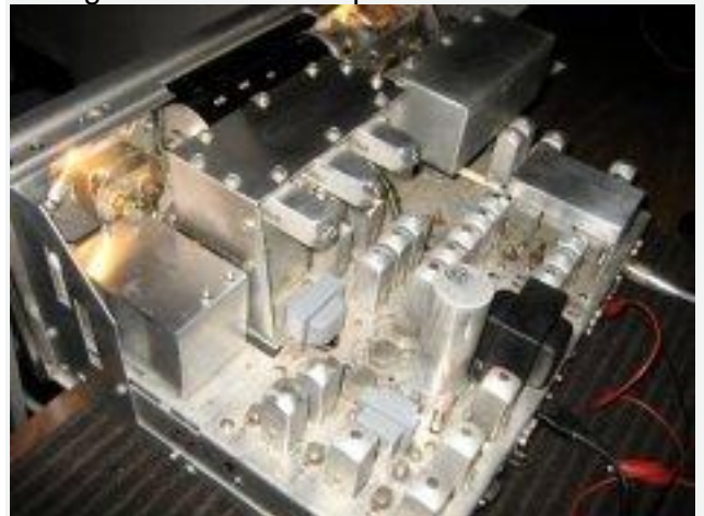
Old capacitors replaced, the cabinet repainted, and power applied. Note the gleaming chassis and components!
