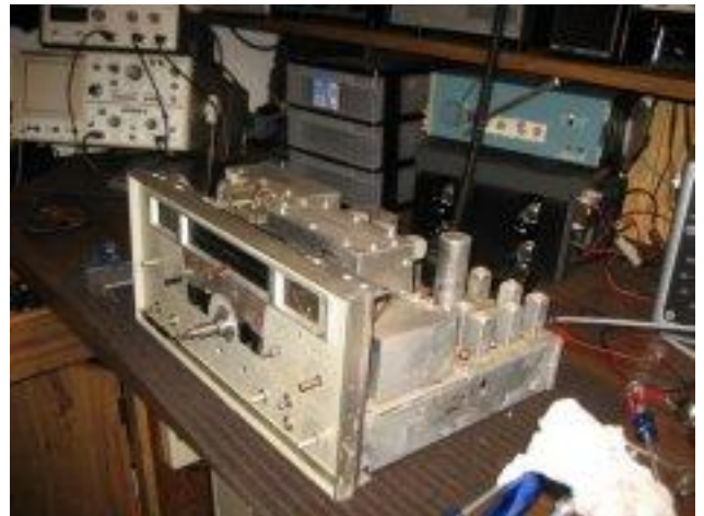
The cabinet is removed and the radio stripped of knobs and other removable items.
