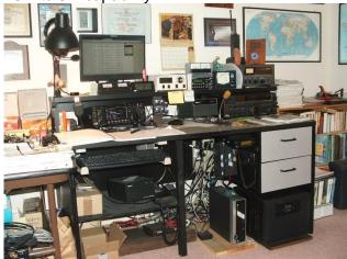
These radios and antennas helped bring Jack's DXCC total up to 350 entities on Phone. On the left is his CW/RTTY station, an IC-7600 driving an ICOM PW1 kw amp (on the floor below the desk drawers). His SSB station is on the right; a vintage IC-775DSP driving a Tokyo Hy-Power HL-1.5KFX kw amp on the shelf above. (Yeah, lots of wires and cables under the desk!)
