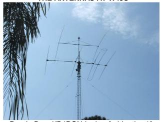
Ron LeBrun-KB4RON is dwarfed by the 40m-6m SteppIR and Cushcraft 40m beam at the QTH of Jack Sproat-W4JS. There's a decent chance the 40m beam will be replaced sometime in the coming Spring with a 7-element 6m beam in Jack's quest for 6m DXCC.
