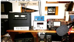
Here are two of the four stations Bob has set up in his shop/garage and house. Here we see an IC-746PRO driving an ICOM PW1 kw amp on 6m. Below the 746PRO is an IC-7600 which also drives the PW1. Bob has a 2m kw amp that can be driven by the 746PRO. Inside his house,
