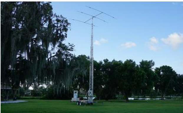
Here's the tower and tri-bander up and in service. A G5RV was used for 40 and 80 meters.
