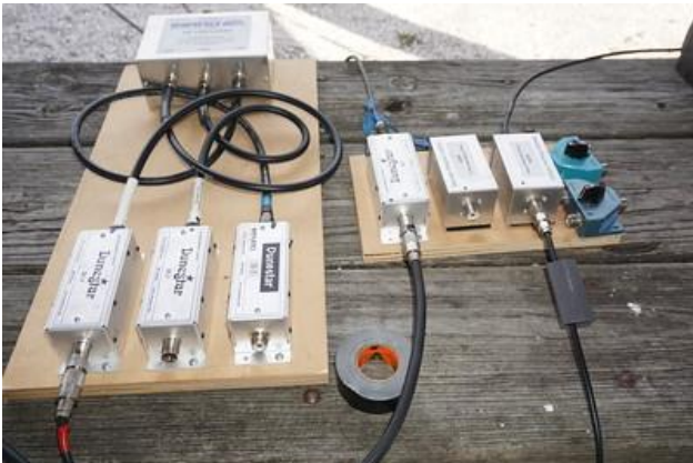
An INRAD triplexer allows the three radios to run all three bands simultaneously to the TA-33.
